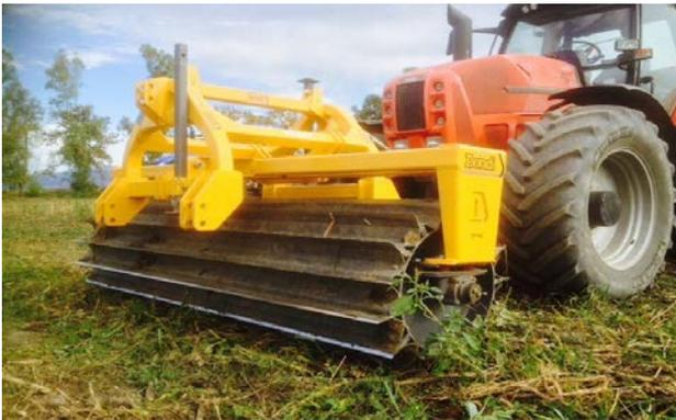
Fig. 3. A roller crimper with blades that can be adapted based on cover crop typology and biomass.
