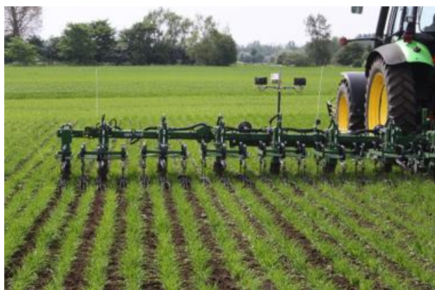
Fig. 1. Inter-row hoeing in spring barley at 25 cm inter-row spacing using vision technology for automatic steering.
