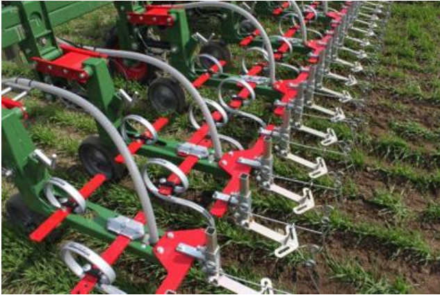
Fig. 2. Parallelograms mounted on a main frame. Each parallelogram is equipped with three hoe shares
