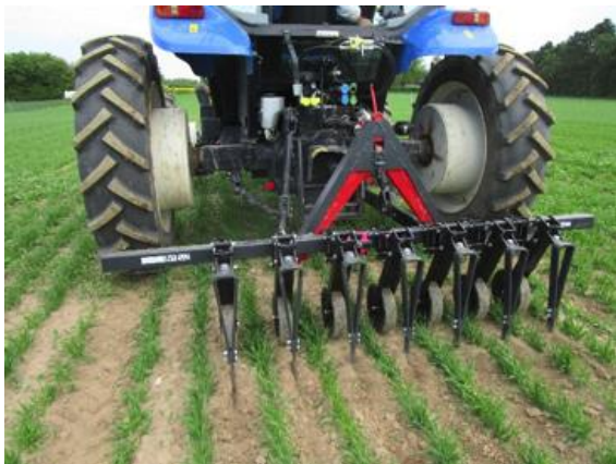
Fig. 5. Operation of the flat hoe share developed by Agrolntelli.
