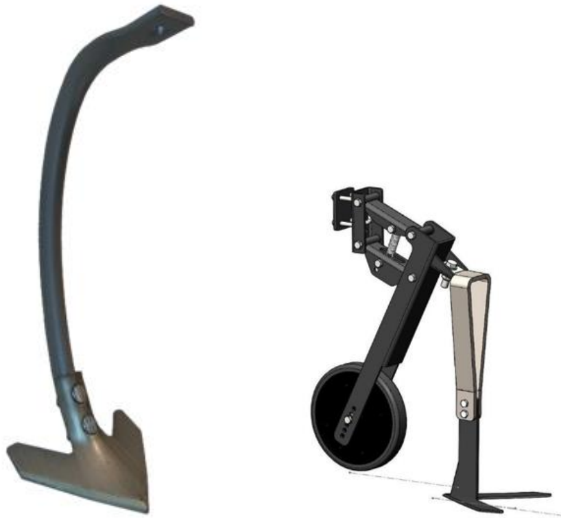
Fig. 4. Ducksfoot-shaped hoe share (left) and flat-shaped share (right). The flat share is developed by Agrolntelli ( www.agrolntelli.com ). Photo credits Liubava Znova.
