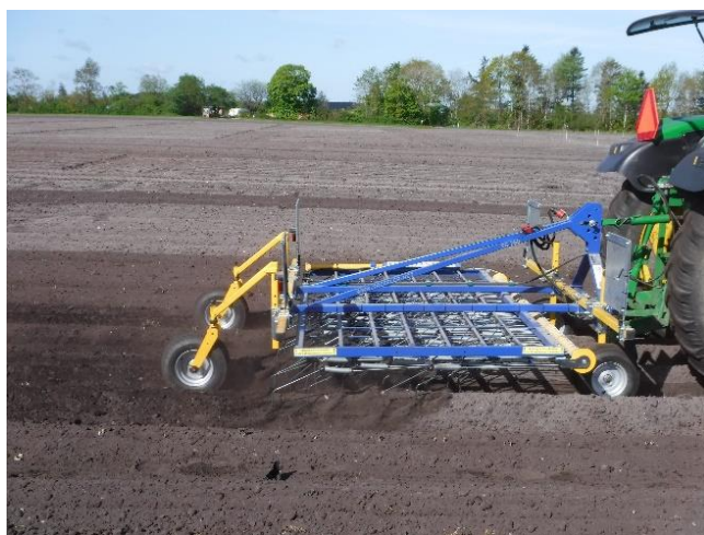
Figure 1. Weed harrowing on potato ridges with Treffler ( www.treffler.net ). Photo: Bo Melander AU
