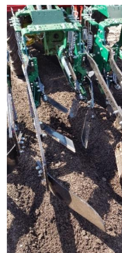
Figure 2. A unit on Optiweeder treating one ridge. Video clips and photos available on: https://msrplanttechnology.dk/optiweeder/fotos-og-video.html . Photo: Bo Melander
