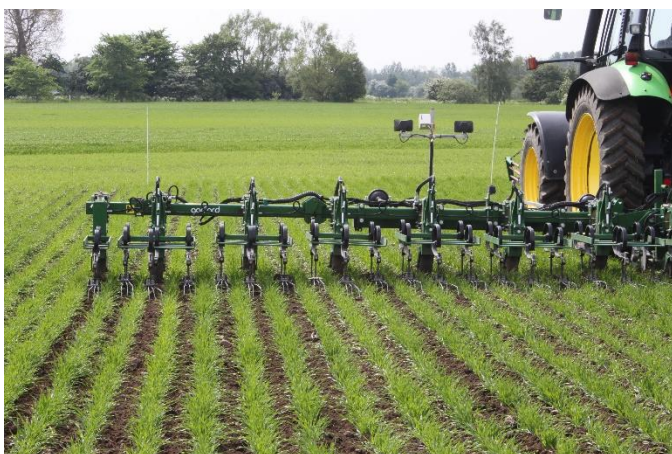
Figure 1. Inter-row hoeing in spring-barley with camera guidance. (Photo: Bo Melander, Aarhus University)
