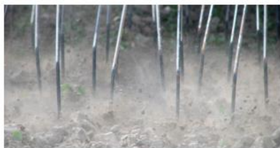
Figure 1 - Flex tines create soil disturbance which causes lethal uprooting and/or soil coverage of weeds. (Photo by Jesper Rasmussen)
