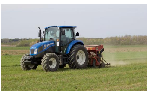
Figure 2. A drilling machine with disc coulters can be used to establish the intercrop in cereals at tillering stage
