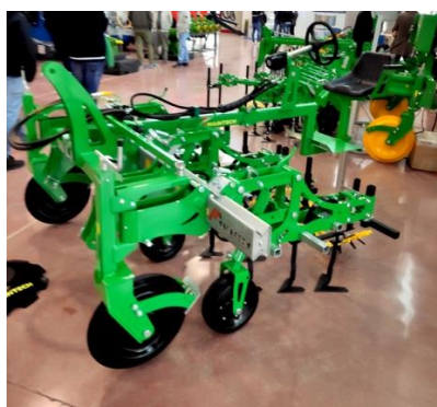
Figure 1. Inter-row cultivator provided with hydraulic assisted manual steering systems
