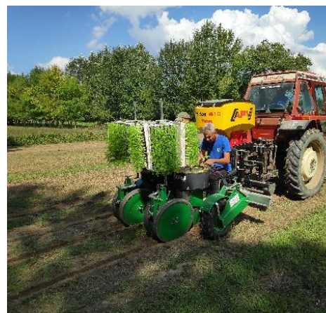
Figure 3. No-till vegetable transplanter equipped with system for localized fertilizer distribution.
