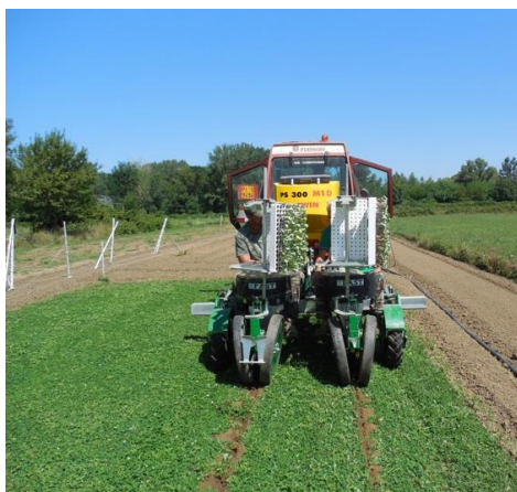
Figure 1. No-till transplanter working on living mulch of “dwarf” white clover var. Pipolina
