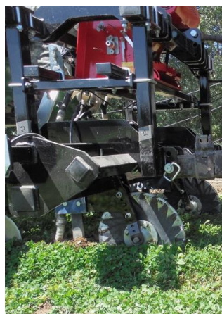
Figure 2. Fluted disc coulters equipped on no-till vegetable transplanter.
