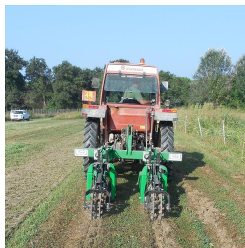
Figure 2. Strip tillage equipment working on living mulch.
