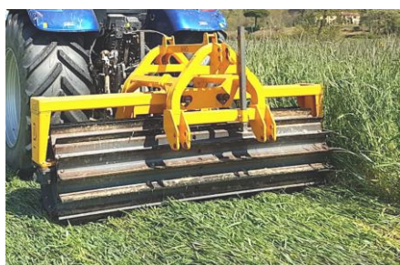
Figure 1. Dondi Cut-Roll RT300 terminating a cover crop of rye.
