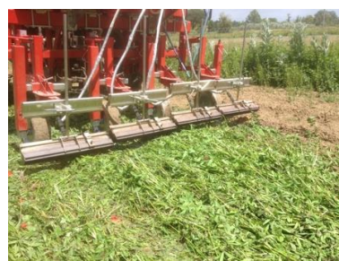
Figure 2. Flame weeding operative machines, working after the roller crimper.
