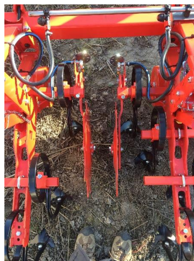
Figure 3. Detail of the prototype showing the herbicide band application apparatus. Photo: Christian Centis, Maschio Gaspardo
