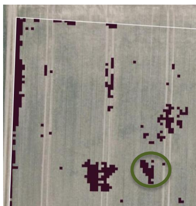
Figure 2. Prescription map from CropManager.dk , 1x1 m pixels for spot spraying of thistle's, dark patches, are the areas that will be sprayed. The thistle patch in the ring is the colony in fig. 1.
