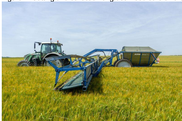
Figure 1. Cutting and collection of grass weed ears on the top of a barley crop. Photo: www.Zuern.de
